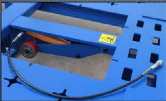
Tilt Deck w/ quick disconnect connection
