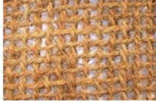
Geo Textiles are a sensible, eco-friendly solution to prevent soil degradation/erosion of embankments, slopes or roads. They are penetrable fabrics having the ability to reinforce, protect, filter, separate and drain. Made from polyester or polypropylene fabric, there are three basic forms - woven, needle punched and heat bonded. The textile lasts for up to 5 years and eventually degrades into humus enriching the soil.
