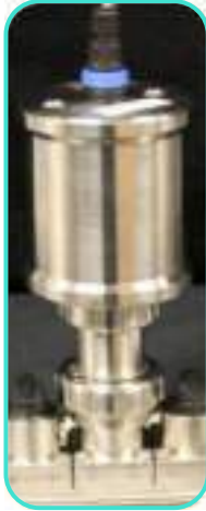
Vapochromic Oxygen Sensor
