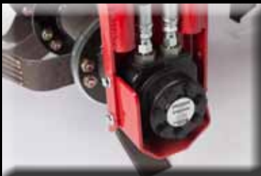
The protected tine motor provides hydraulic direct drive to the shaft
