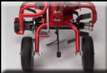
Tilling depth can be adjusted by setting the wheel height
