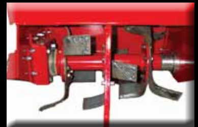
Hard faced, counter-rotating tines cut through sod and hard packed soil
