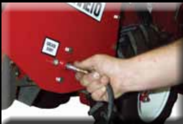
Marked grease zerks allow for easy maintenance
