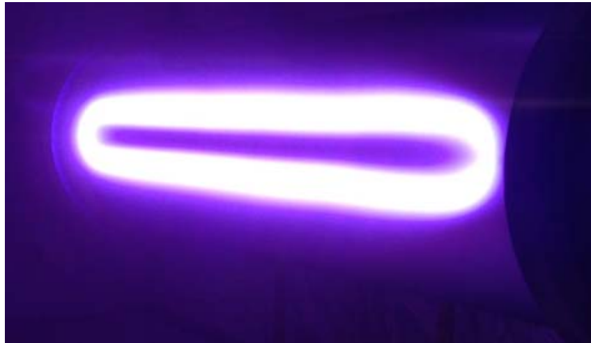
Figure 3. Uniform Magnetic Field Racetrack Plasma on Rotary Magnetron
