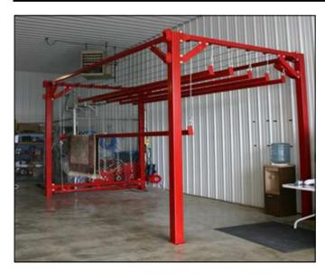
**Rug Drying Tower - Powered** uses a winch & pulley system to raise wet rugs for drying.
