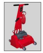
Mini Rug Duster Cub weighs 65 lbs, has a ½ HP motor and an adjustable handle. It has a 15" cleaning path. The 15 double ended vibro straps rotate counter clockwise at 15,000 vibrations/minute. No vacuum port is included.
