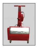
Rug Duster weighs 90 lbs, has a 1HP motor and an adjustable handle. It has a 25" cleaning path. The 25 double ended vibro straps rotate counter clockwise at 47,000 vibrations/minute. A vacuum port is included for dust collection & environmental safety.
