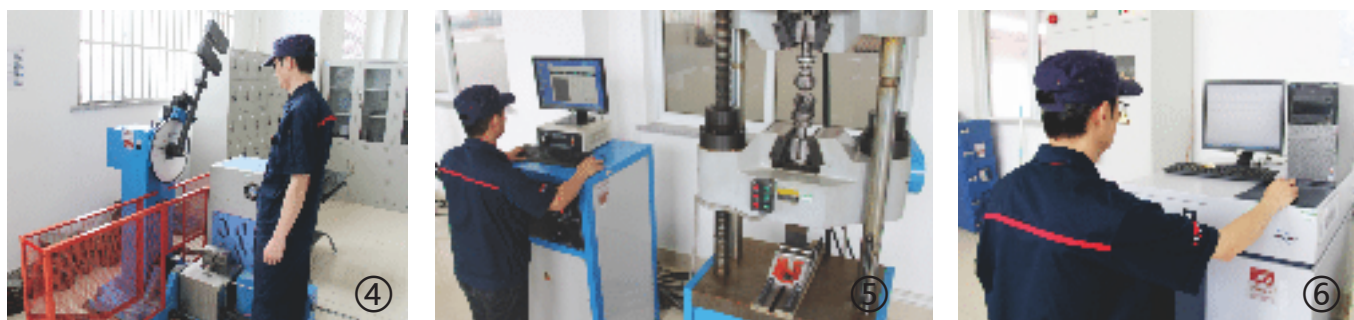
④ Impact testing machine are necessary in testing mechanical properties of the products and impact value of KA.
