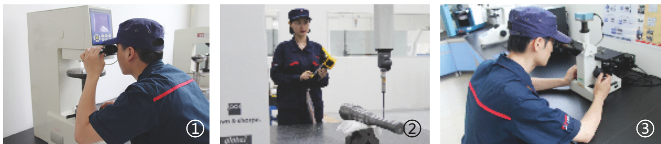
① Rockwell hardmeter can be used to test material samples' Rockwell hardness(Left). Brinell hardness tester can be used to test material samples' Brinell hardness.(Right)
