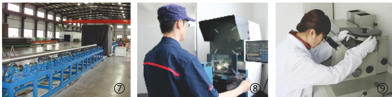
⑦ Magnetic powder flaw detector provides surface inspection of material with fluorescent magnetic particle. It detects and highlights any defects on the surface.
