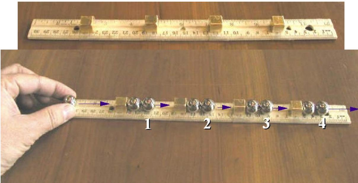
**Figure 1. Gauss Rifle set-up recommended by Science Toys.**
