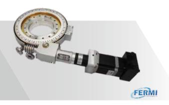
This device allows UHV equipment to be rotated about the flange axis for concentric polar (eucentric motion about the flange axis). Applications include sample imaging(XPS, AES or SIMS), structural or ion/neutral/atom scattering experiments.
