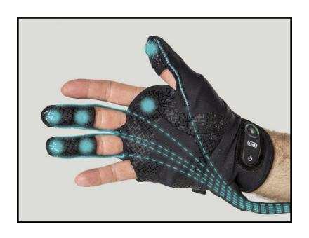
Picture shows a black glove showing pressure sensors worn on right palm of a hand
