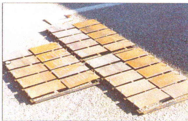
Fig. 1: Panels waterjetted to a WJ-2 condition
