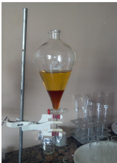
Fig. 2. Separation of sesame ethyl esters and glycerin
