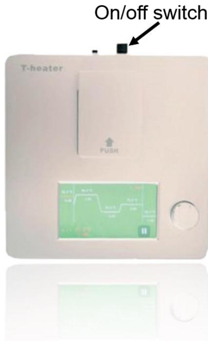
11. Enter the settings indicated in step #9. To change a setting, first tap it on the touch screen and then adjust its value by turning the rotary knob clockwise (to increase) or counterclockwise (to decrease).
