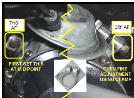
Figure 14 Distributor adjustment
