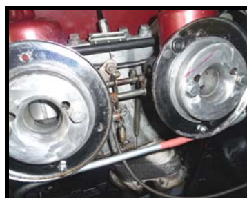
Figure 34 – Carburettor Overflow Pipes
