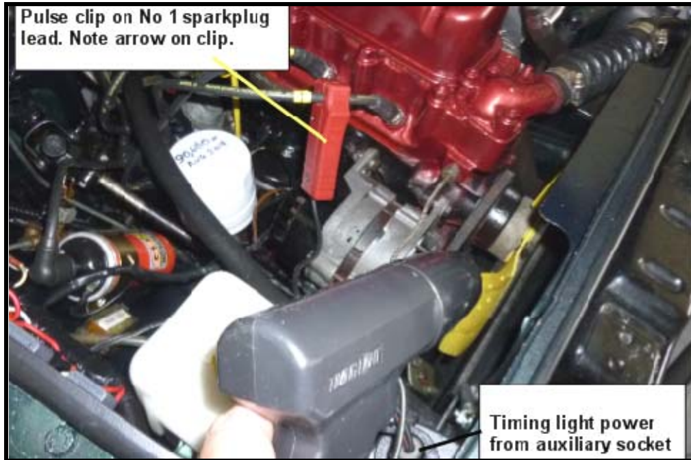
Figure 17 – Timing Light Setup
