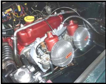
Figure 27 – Dual SU HS4 (1½”) Carburetors
