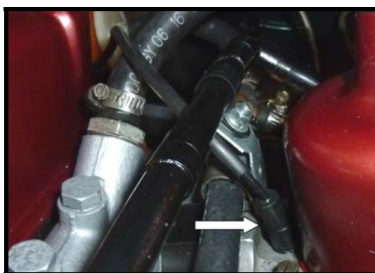
Figure 8 – SU Carburettor Vacuum Advance Connection
