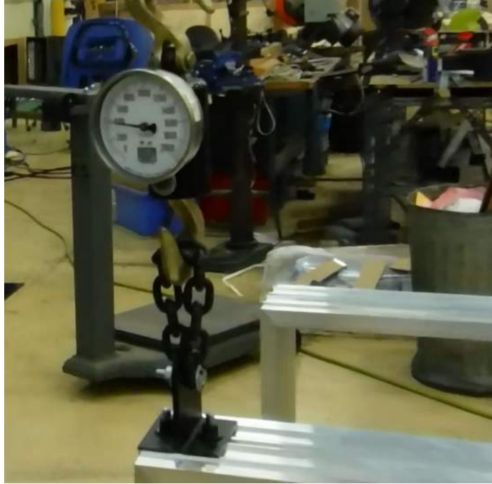
Photo 2: Test LT-2, Side Frame Connection Test [400 LBS]
