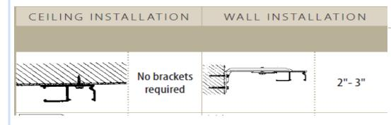
Track perforated 16" on center for direct mounting with screw. Wall Mount:
