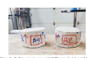
Figure 2 - Roofing concrete cores with MVRA, samples A-1 and A-2.
