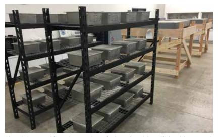
Photo 2: Concrete slabs and pan specimens, both regular weight and lightweight structural concrete, in SRI Consultants' laboratory in 2016
