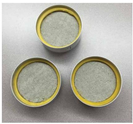
Photo 5: Concrete specimens prepared for ASTM E96 water vapor transmission testing
