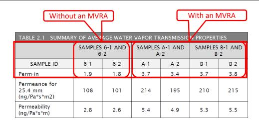
The specimens containing an MVRA have tested WVT values about two times (i.e., more "vapor open") more than the specimens without the MVRA
