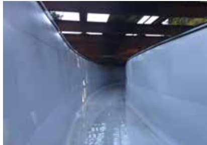
PHOTO 5 Testing flume with water after completion.
