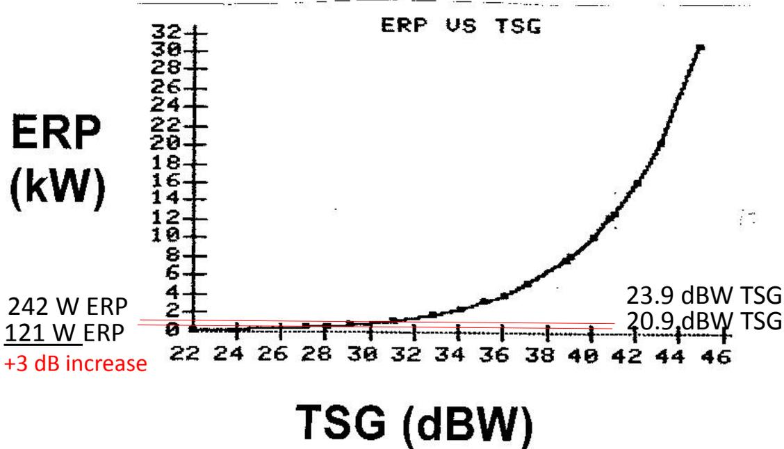
As transmit system gain increases, ERP improves exponentially; and big gun HAM stations can easily reach above 12 kW ERP
