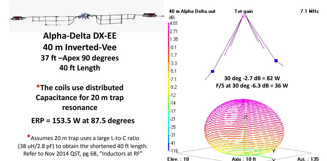
Alpha-Delta DX-EE Inverted-Vee Large Coil results in higher losses and narrower SWR bandwidth SWR between 7.0 and 7.3 MHz
