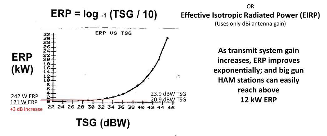
**ERP Is Calculated to Show the Equivalent Power in the Best Antenna Direction**
