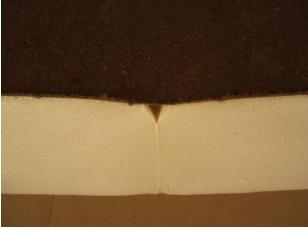
Knit line and V-groove close-up (after conditioning)
