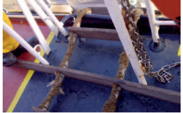
Poor and incorrect securing method
