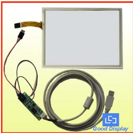
8inch Touch Panel and USB Driver board
