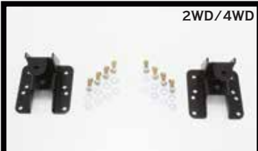
Rear Lift Hangers (w/ Flip Kit raises the Back to 5" or 6") (#93049)
