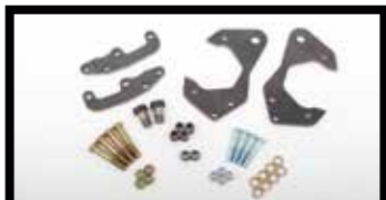
Front Disc Brake Brackets - Use Rotor Kit #63201. Moves wheels out 3/4" on each side. Will not work w/ Factory 14" wheels. (#63228)
