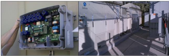
Fig.1: Inverters: small-scale inverter box for residential use (left) and Satcon utility-scale inverters (right)[2]
