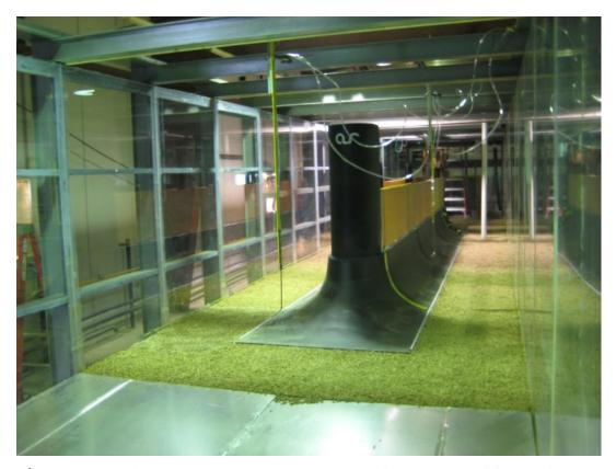
Figure 8. Photo from upstream of the AUR full-scale 10.16m long 1.42m wide  $\text{scAUR}^{\text{TM}}$  with  $\text{VorGAUR}^{\text{TM}}$  vortex generators model in the IIHR Environmental Flume Facility with three 2.44m side sections on each side for Configurations A and B. Small and large gravel on opposite sides are flush with the edge of the model.
