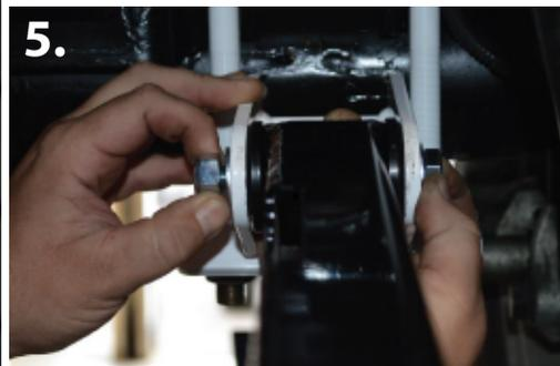
7. Now install provided bushings and sleeves in the traction bars.
