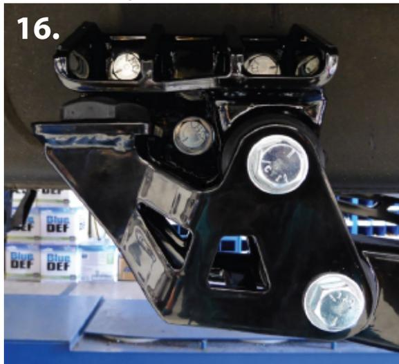
20. Now fully assemble shackle and traction bar back onto the frame mount. (pic 16)
