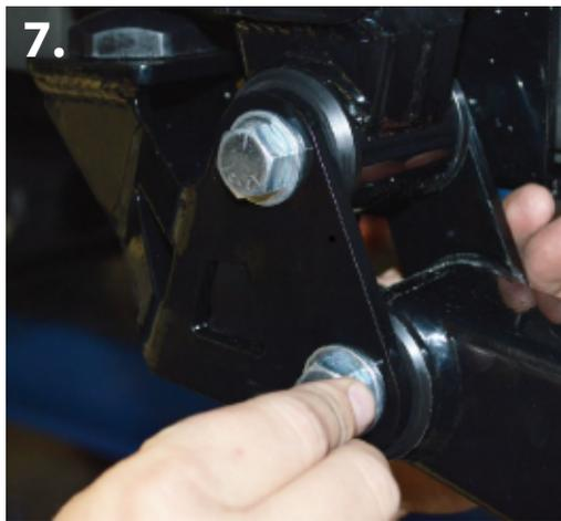
9. Assemble shackles and frame mount brackets with provided bump stops, bushings, and sleeves.
