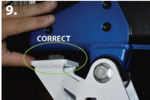
12. With the brackets fully assembled, lift the frame mount up and place against the bottom of the frame. Making sure there is no gap between the bump stop and the frame mount.
