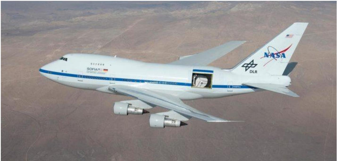
Figure 1 – NASA's SOFIA airborne observatory with telescope visible in the observing portal. (NASA)
