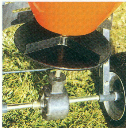
Reversible spreading disk. Same distribution independently of the working direction.
