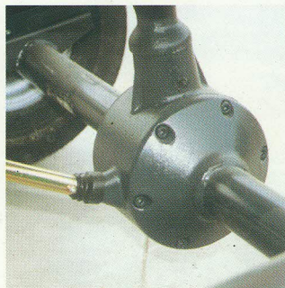
Strong gearbox with disengaging lever.
