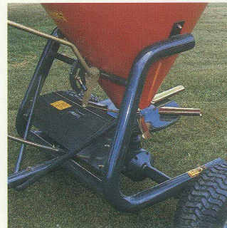
Strong tubular frame overdimensioned to resist tensions even with the hopper filled up while driving.
