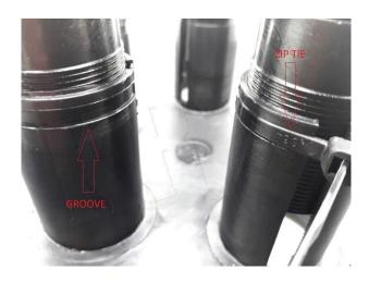
5. Reinstall the cap assembly again and wheel is complete. If you want to install the caps on a different wheel at a later date, you will need to remove the zip ties to allow the cap and bracket to be adjusted to fit the new wheel.
