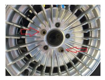
2. Look at the mounting bracket and observe the 2 holes that are larger than the others. These will be installed over the first 2 lug-nuts. While holding the bracket in place on the wheel, install the 3 flanged bolts that are supplied with the order, securing the bracket to the car: do not torque these down yet, as you will be removing the bracket shortly.
