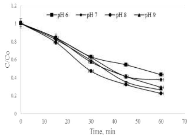
Fig. 2. Effect of pH on dye degradation using co-doped ZnO
