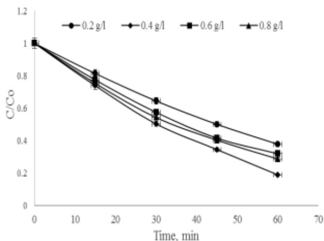
Fig. 4. Effect of catalyst loading on dye degradation of doped ZnO
