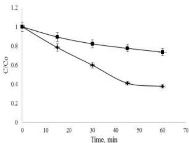
Fig. 1. Effect of dye degradation for co-doped (◆) and undoped ZnO(■) catalyst
