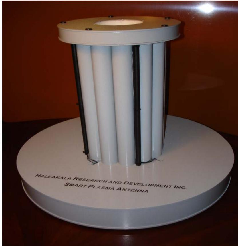
**Haleakala R&D, Inc. ruggedized smart plasma antenna prototype.**
