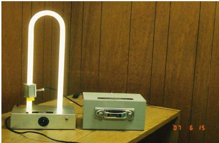
**Plasma Antenna for AM/FM Radio Prototype. This is on display at the Booz Allen”
