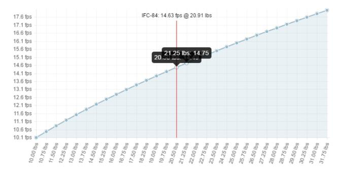
The above graph indicated the associated weight, in lbs, to the descent rate, in ft/s, depending on the type of parachute and the weight of the rocket.
