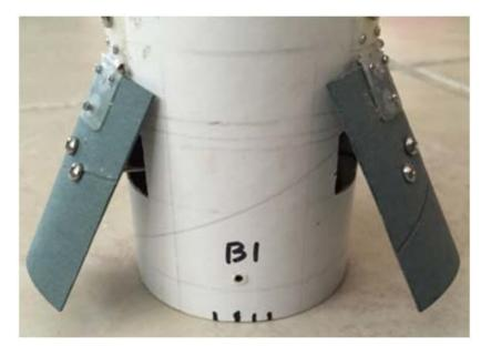
The air brakes will be used for controlling the altitude of the rocket through drag rather than
