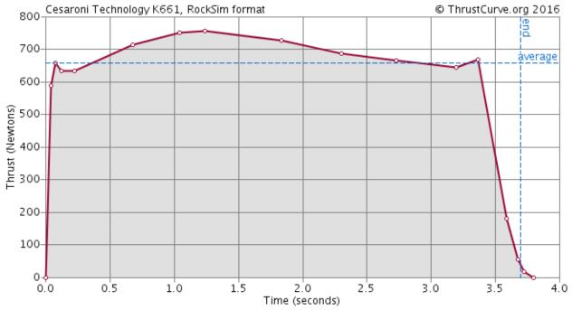
Even though the simulated altitude with a Cesaroni K661 is well over 5280 ft, the air brakes should adjust to bring the rocket down. Other motors were eliminated because they did not fit the 75 mm diameter motor mount and/or caused the rocket to fly too high.
