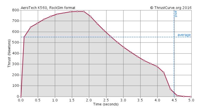
Although the Aerotech K560W(thrust curve pictured above) was considerably closer to the altitude, it did not have this "spike" in its thrust curve. The below thrust curve of the Cesaroni K661 does.
