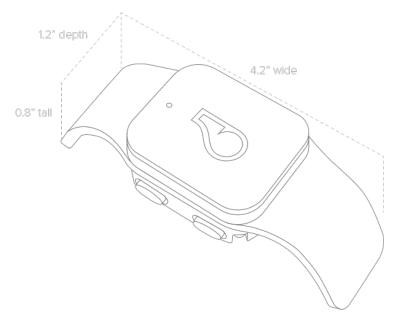
It has the dimensions of 4.2" x 0.8" x 1.2" with a mass of 35.44 g, with a battery life of up to 10 days of continuous use. The dog collar will simply be placed into the rocket after being charged from the base station, and no other technical interference is necessary to activate it. The base station, or the charging station of the Whistle GPS, is seen in the following diagram:
