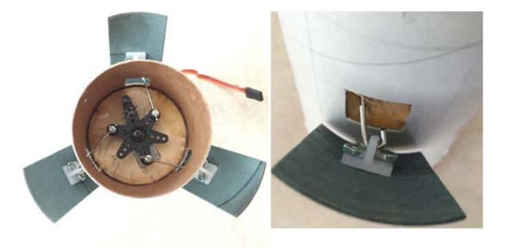
The above three pictures are of the TARC rocket's air brake module.
