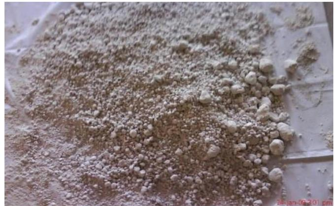
Fig.1 – Raw Hypo sludge disposal from TNPL
