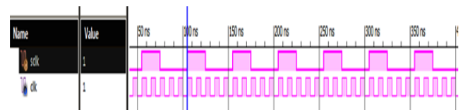
Fig. 6.1: Generation of clock signal of 20 MHz
