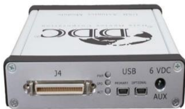
Fig. 4.1: USB port facing of the DDC module
