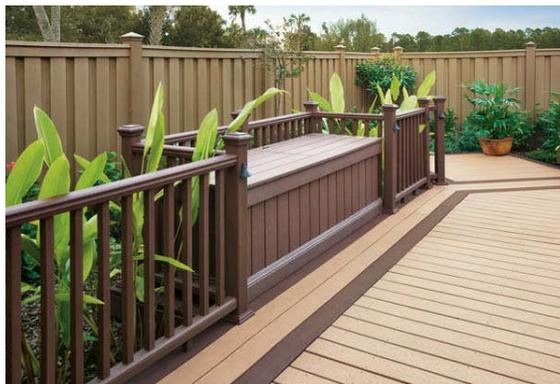
Trex composite fencing is made of recycled plastic and wood. The company buys 300 pounds each of landfill-bound polyethylene and hardwood sawdust annually.
