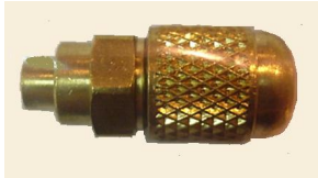
Schrader Fitting Body, 1/4" Male Flare, Braze-in
