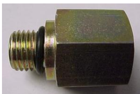
Male 7/16-20 Straight Thread O-Ring x Female 1/4" NPT
