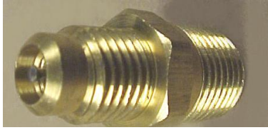
Fitting, Male 1/4" NPT X Male 1/4" Flare Access Port with Schrader
