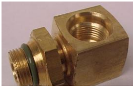
90 Elbow Swivel R134A Male M13 Straight Thread x Female M13
