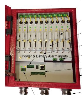
Opto-Channelized <sup>TM</sup> cards 1 frequency per card, ´any band, individual channel control
