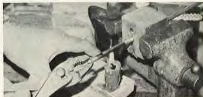
Heat from candle softens ferrule cement and lets you remove points from aluminum shaft.
