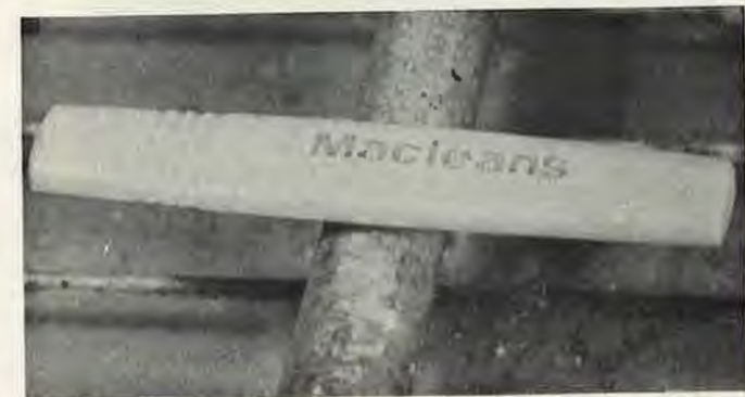
Toothbrush is trimmed to size of rest desired (top), then surface roughened and contact cement applied. Squared-off remainder of handle (below) is then set atop metal rod or large bolt placed in the oven.
