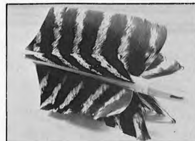
Inspecting the fletch from the side, one can see that edges are left untrimmed. Only the back section of the nock has been trimmed to keep even on the shaft.
