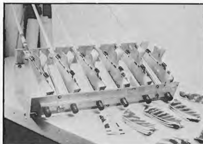
After trimming end of fletch, put it in the clamp, then apply cement down the quill. Set indicator nock on jig for the first station, then place the clamp in position.
