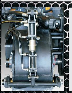
Unique to the **TRANSFORMER GRINDER** dual cylinder depth control system. This system was designed to make removing skip lines on the highway much simpler.
