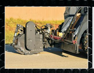
The **TRANSFORMER GRINDER** incorporates tool pivot mount that allows the tool to follow any contour the surface may have. combine the tool pivot with the glide wheel depth control and you have a grinder that is unsurpassed in the consistency of the cut.
