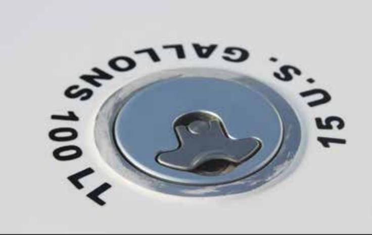
The XS we flew holds 15 gallons of fuel per side. Current kits hold 20 gallons per side for a total of 40 gallons, with 38 usable. Unlike the old tanks, the new tanks are removable for servicing.
