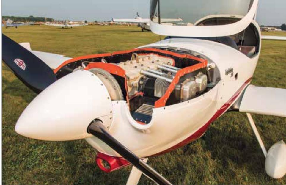
It's the larger Lycoming O-320 that turns the LSA Lightning into the Lightning XS, but the 160-hp UL Power engine is also available.
