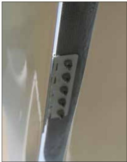
The elevators use simple, top-mounted hinges to attach them to the stabilizer. Control feel is quite good.
