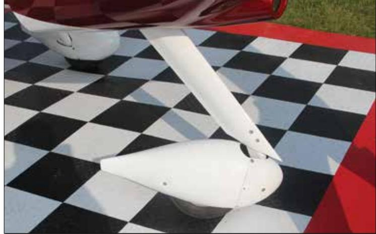
The free-castering nosewheel is typical of small tricycle-gear homebuilts and provides tight maneuvering on the ground using differential braking.
