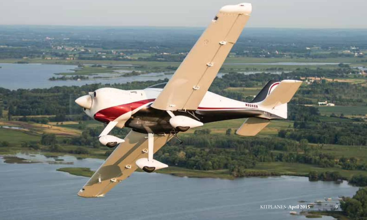
for Arion by a subcontractor (Fiberglass Molding of Weyauwega, Wisconsin), and the builder can start with something that looks very much like an airplane, right out of the box. The XS has a different cowl to enclose the larger Lycoming engine, but aside from that, it is hard to tell the difference between it and its LSA forebears at a distance. The composite used is a vinylester resin, rather than epoxy, chosen by Otterback for its strength and light weight.
