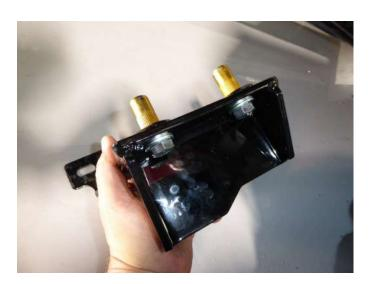
18. With both holes drilled out, insert the two provided 1/2" bolts into the frame bracket with the provided rivet nuts installed.
