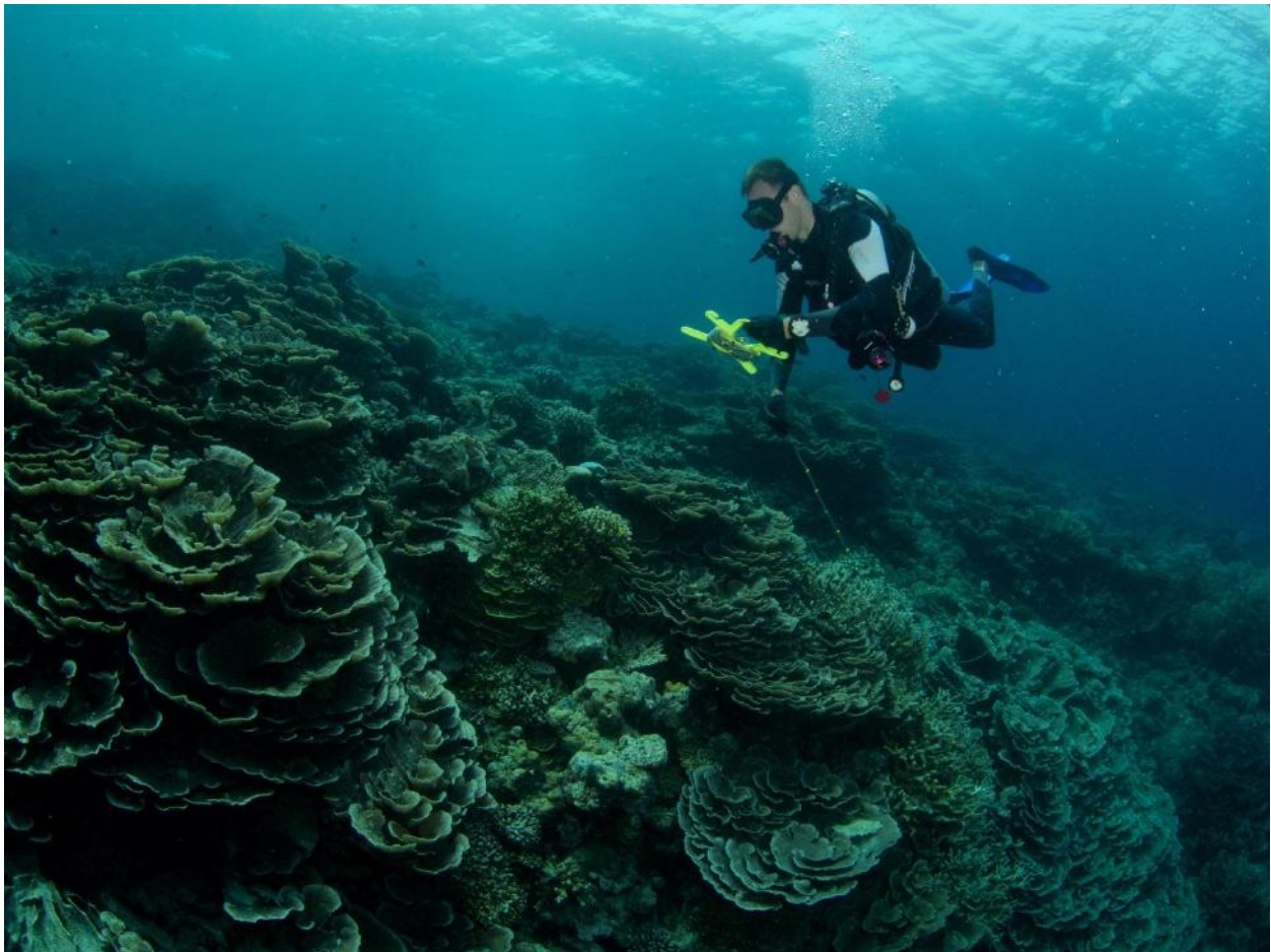
Fig. 3. Deploying a 10 m lead line at 10 m depth. Each line is marked with 100 points.
