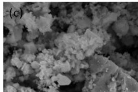
**Figure. 2 SEM images of Mn doped SnO<sub>2</sub> (a) 2% Mn Doped SnO<sub>2</sub> (b) 4% Mn Doped SnO<sub>2</sub> (c) 6% Mn Doped SnO<sub>2</sub>**
