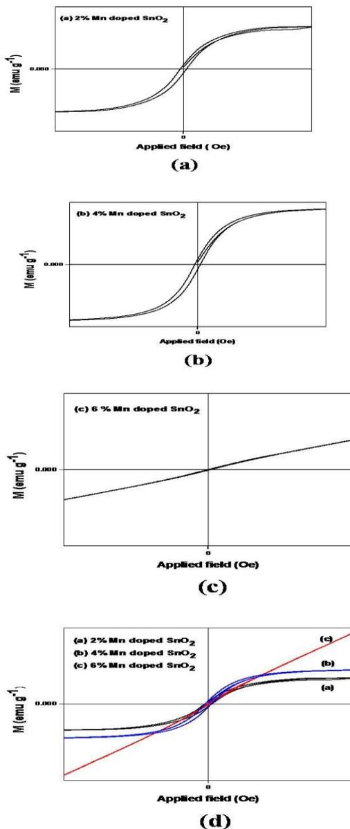
**Figure.3 Magnetisation curve of (a) 2% Mn Doped SnO<sub>2</sub> (b) 4% Mn Doped SnO<sub>2</sub> (c) 6% Mn Doped SnO<sub>2</sub> (d) Comparison of 2%, 4% and 6% Mn Doped SnO<sub>2</sub>**
