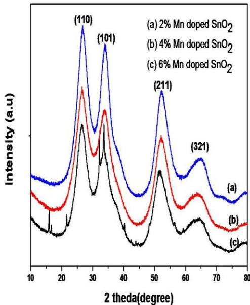
**Figure. 1 XRD Pattern of (a) 2% Mn Doped SnO<sub>2</sub> (b) 4% Mn Doped SnO<sub>2</sub> (c) 6% Mn Doped SnO<sub>2</sub>**
