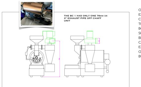
ONLY ONE EXHAUST PIPE COMES OFF THE BC-1 AT 3" AS SHOWN BELOW AND CAN BE EXHAUSTED OUT OF BUILDING.
