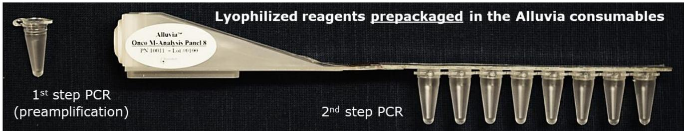
The Alluvia consumable can be used as a vehicle for ready-to-use PCR assays, especially 2-step PCR assays. The system minimizes pipetting steps, provides continuous sample containment, and interfaces with standard instrumentation.
