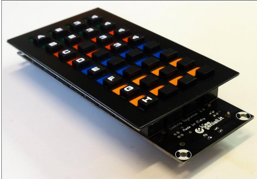
Coding spacemat has 32 working keys and a USB-B connector. Device is self-powered by USB port. Please connect to a PC with a USB A/B cable (sold separately). Keyboard is auto-detected within a few seconds, it doesn't require any special driver in most common operating systems: Windows, Linux, Mac, Android.
