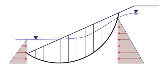
Figure 3 – Seepage Forces with Pond
