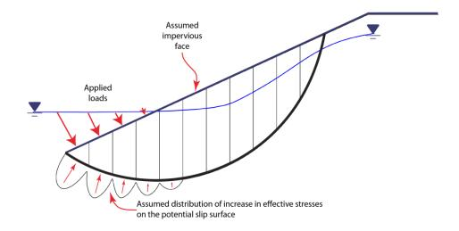
Figure 4 – Application of Pond Pressures
