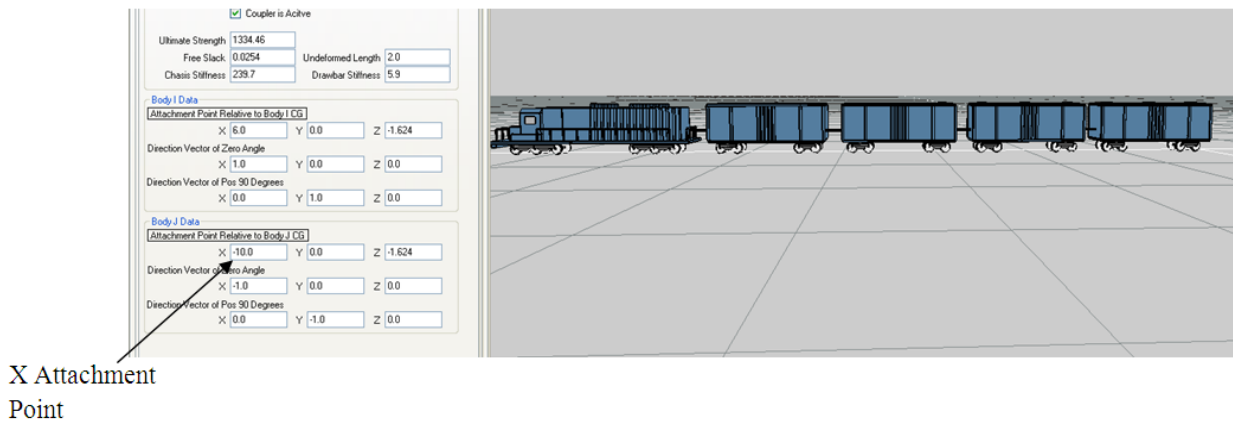
Fig. 4.12 – Local Coupler Attachment Point On Locomotive
