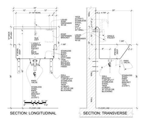
Engineering Specification: 14 gauge, type 304 stainless steel wash sink.1-3/8" rolled rim. 1-1/2" welded in drain. Exposed surfaces polished to a satin finish. Supported on (2) wall clips.
